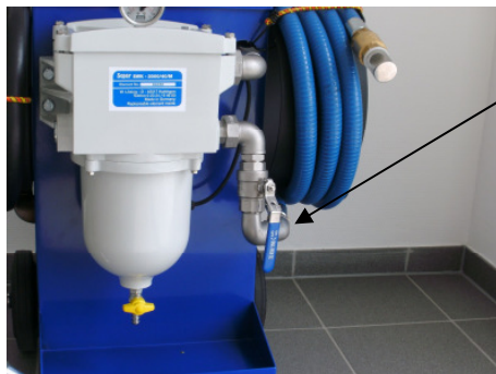
Shut off valve opened
